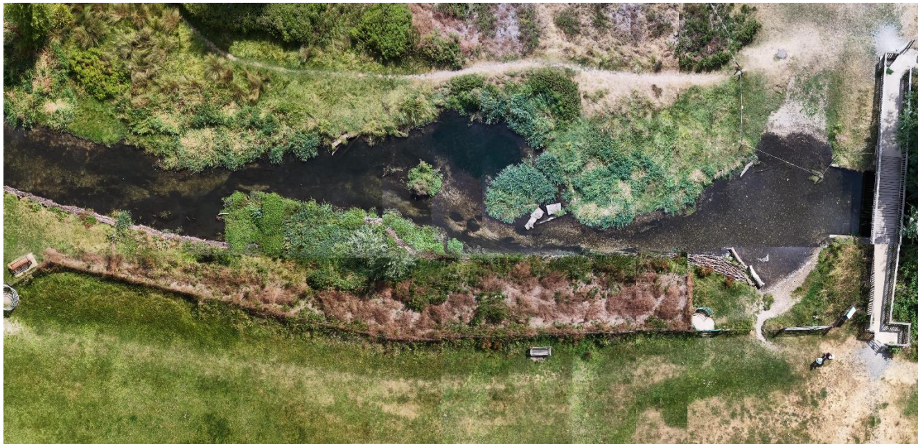
Image 5: High-resolution 2D orthomosaic map of the River Bulbourne restoration site, generated entirely in-browser using PostFlightStudio to allow monitoring of chalk stream channel health, marginal habitat growth, and in-stream features.
